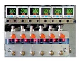
The air+oil flow is continuously controlled by precise opto-electronic sensors which can detect changes in lubricant quantity and air-flow giving immediate signal to the PLC of the control unit. Mixer type MVF-A is available in versions from 1 up to 6 outlets.
