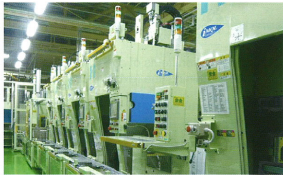
Fig. 6: Mission case machining line thoroughly with iMQL ® (NS70 as machining unit.)
