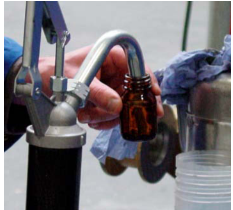
Figure 3 Lubrication requirement for a work shift using MQL
