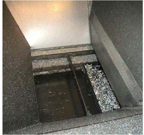
Figure 32 Chip conveyor as extraction position
