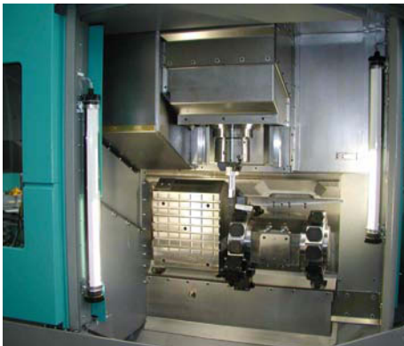
Figure 21 Inner view of an MQL machine tool
