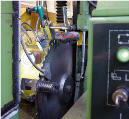
Figure 52 Sawing with minimum quantity lubrication
