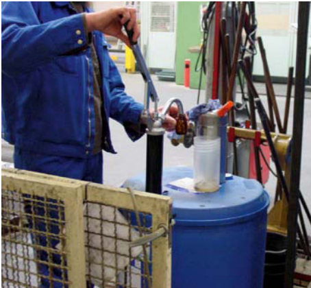
Figure 2 “Central lubrication store” for minimum quantity lubrication
