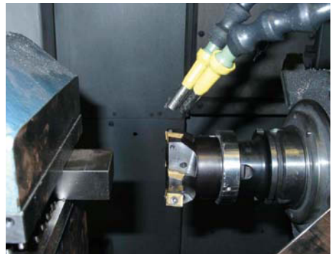
Figure 5 External feed via nozzles
