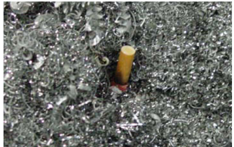
Figure 51 Burning cigarette butt in the chip container
