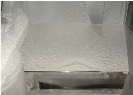
Figure 48 Sticky mass in the machine interior
