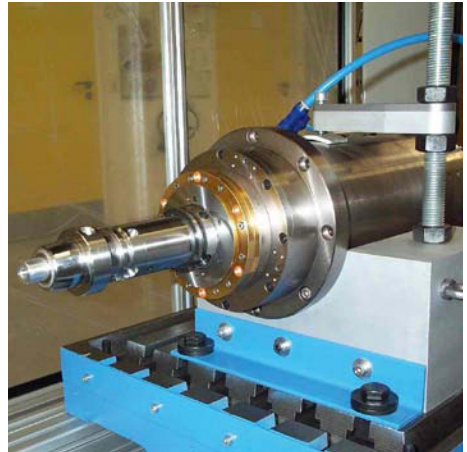
Figure 45 High-speed spindle with internal feed (30,000 rpm)
