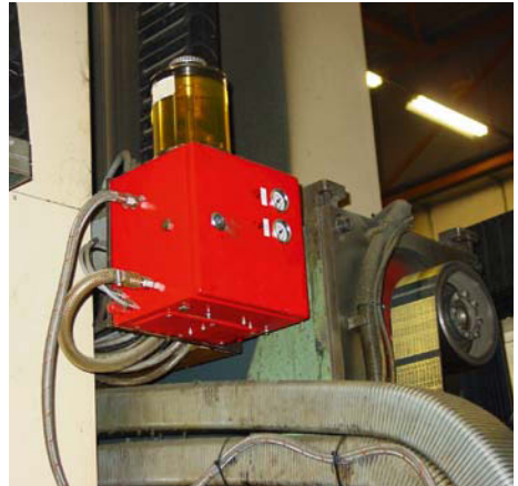
Figure 55 Clean lubricant with MQL system
