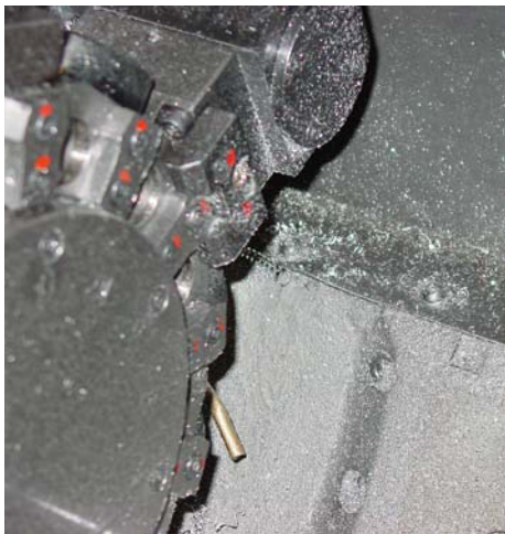
Figure 33 Chip accumulation in corners and edges
