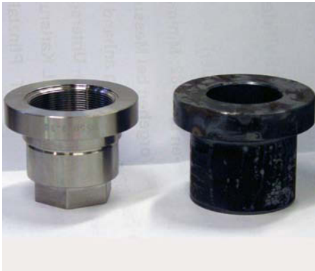
Figure 42 Machined revolver nut and unworked piece; material: CK 45
