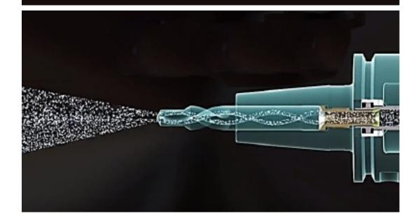
MQL systems for tools lubrication from inside with lubricant supply through spindles, revolvers and tool holders for
